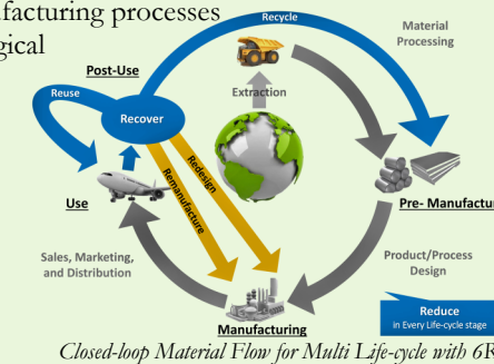
Closed-loop Material Flow for Multi Life-cycle with 6Rs
