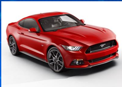
Ford Mustang : Aluminum hood, Aluminum fenders & aluminum engine with composite coated Cylinder bores
