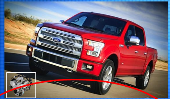
F150 - Aluminum Body, Closures and Truck bed, UHSS Frame
