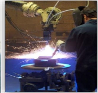
Aluminum brake rotor with thermally sprayed wear resistant coating
