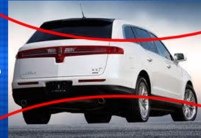
2010 Lincoln MKT : Light- weight magnesium and aluminum lift gate.
