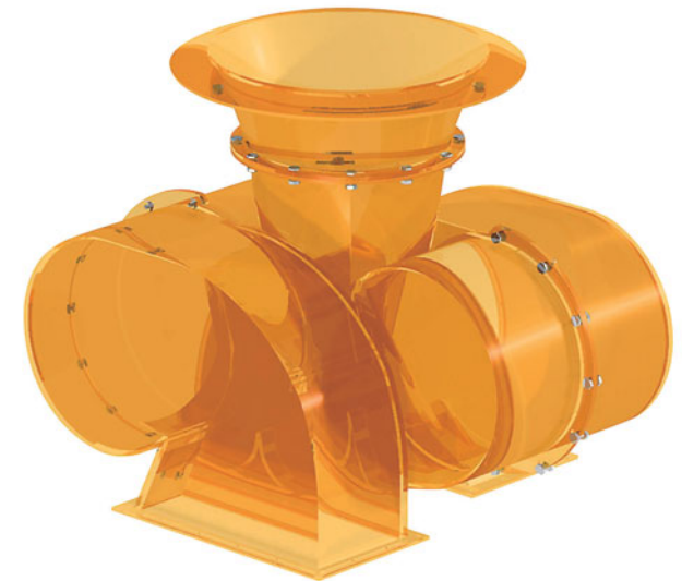
Vortecone Scrubber, an over-spray paint capturing device, developed by Dr. Saito (in cooperation with the University of Kentucky, Toyota Motor Corporation, and Trinity Industrial Corp). Patents have been obtained in the US, Europe, and Japan.
